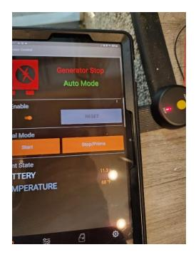
3.Click the AGS Enable toggle button – AGS Switch LED ON  $\rightarrow$  AGS module and AGS switch are communicating.
