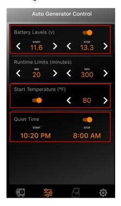
Check the settings conditions for operating the generator with AGS, such as temperature, voltage, and whether quiet time is enabled.
