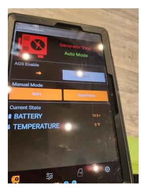
If the AGS app is in the Enable state but the LED light on the AGS switch does not turn on and the temperature from the temperature sensor is not displayed on the app, it is highly likely that the switch is not properly registered.
